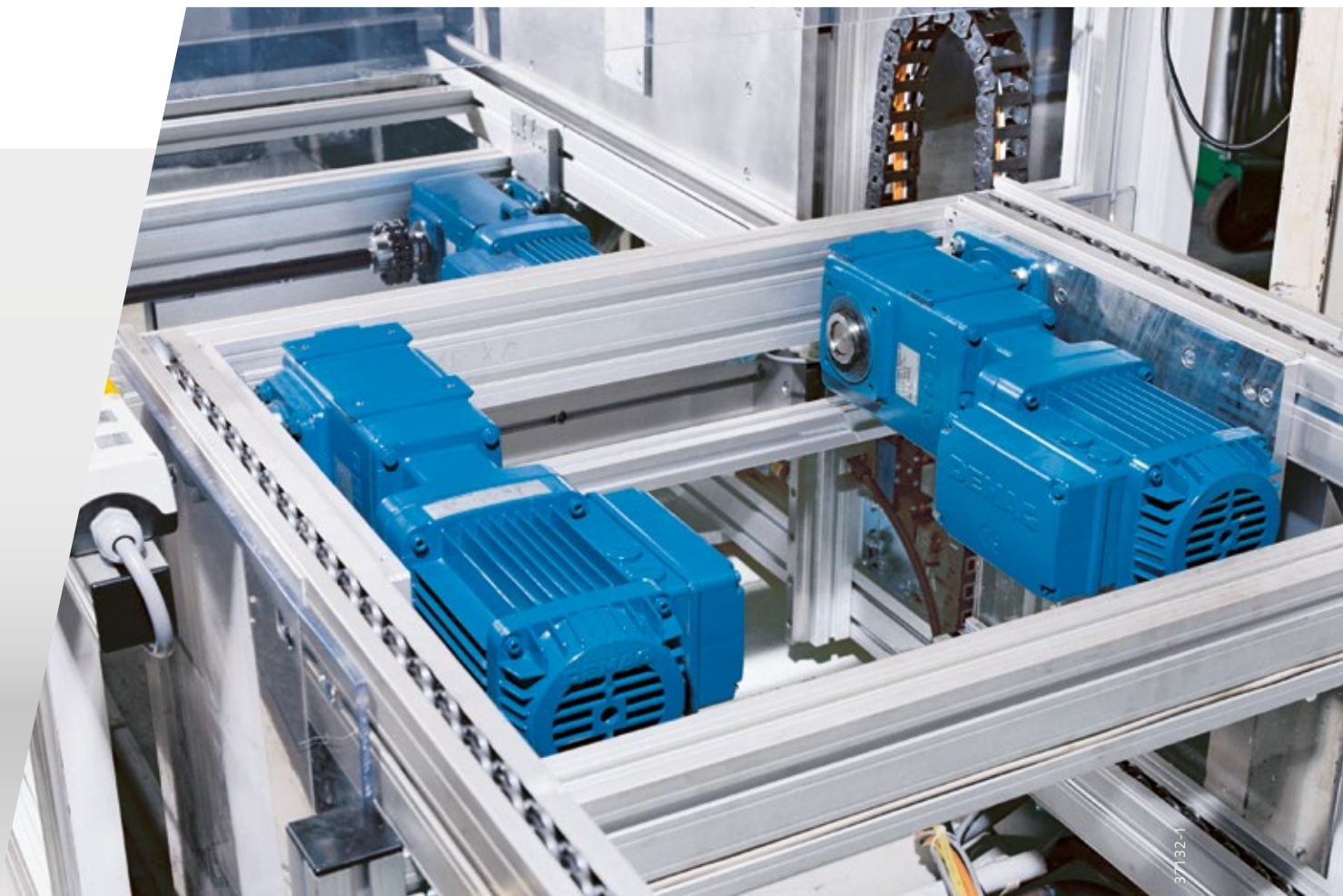
Angular geared motors for compact drive solutions.
